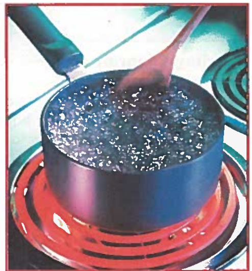
▲ The wires in a burner slow down electric current so much that the burner gets hot and glows.
