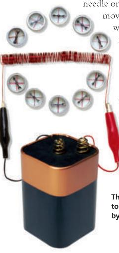
needle on a nearby compass had moved. Oersted realized that a wire with electric current flowing through it creates a magnetic field. The magnetic field around the wire acts as an invisible magnet. This is why the compass needle moved.
